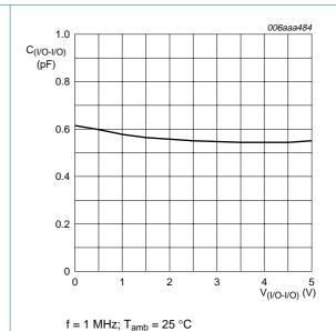
Fig 3. Input to input capacitance as a function of input to input voltage; typical values
