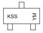
$$\begin{split} & \text{KSS} = \text{Product Type Marking Code} \\ & \text{YM} = \text{Date Code Marking} \\ & \text{Y} = \text{Year ex: N} = 2002 \\ & \text{M} = \text{Month ex: 9} = \text{September} \end{split}$$
