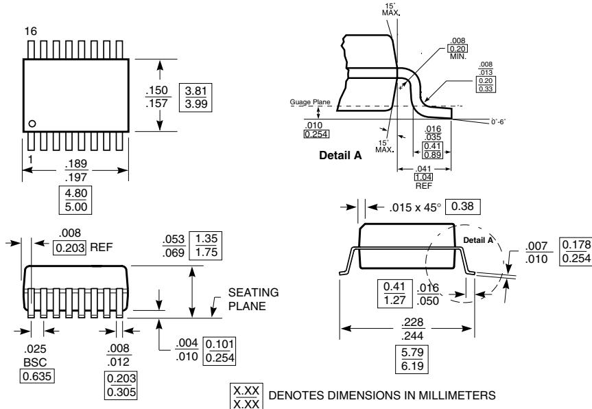
**Packaging Mechanical: 16-pin SOIC (S)**
