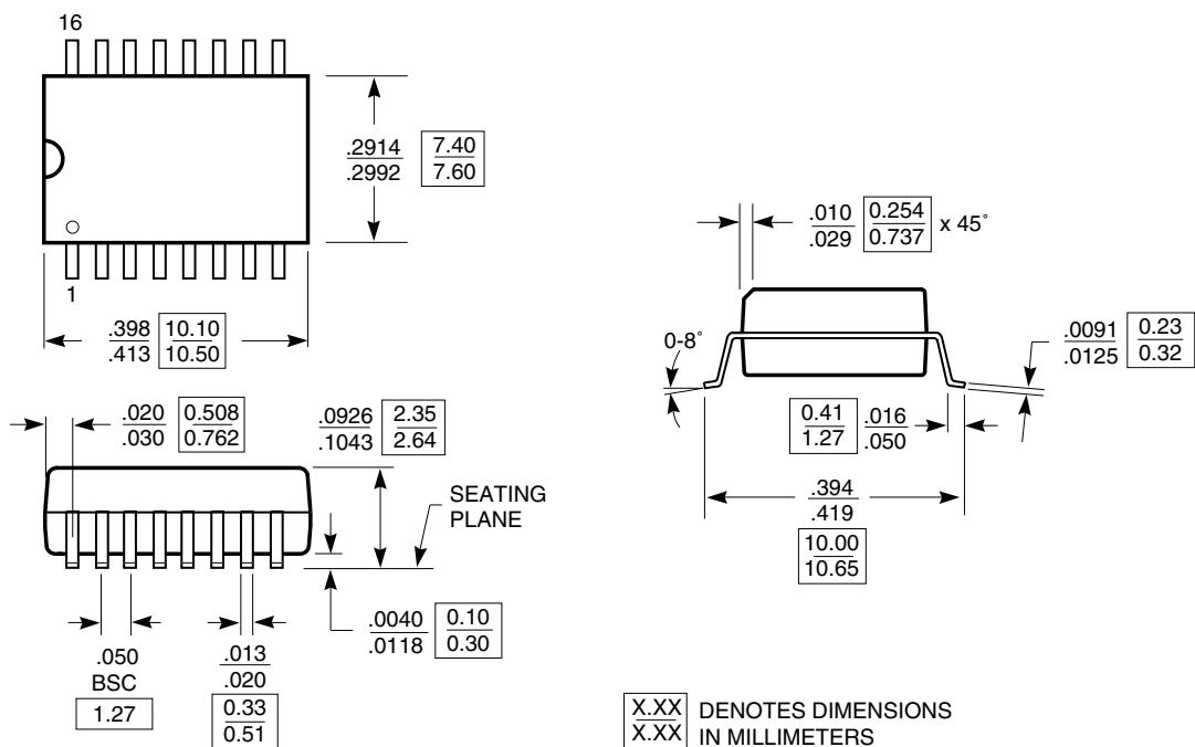
**Packaging Mechanical:16-pin SOIC (W)**
